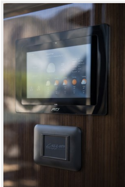
RTI lights and curtains automation
