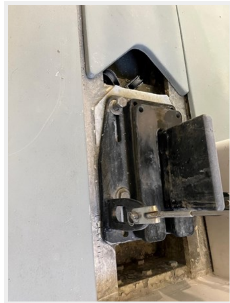
Mast step IMG_1852
