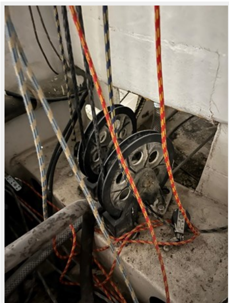
Steering cables sheaves IMG_1847
