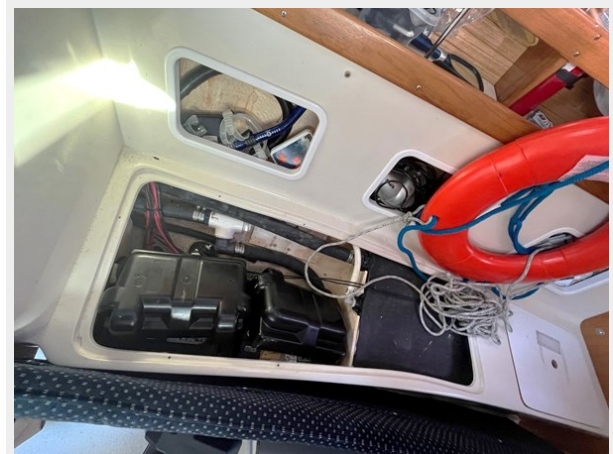
Batteries & Holding tank IMG_1759
