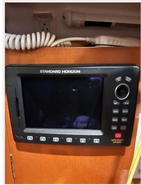
Std Horizon CP300 GPS plotter IMG_2093
