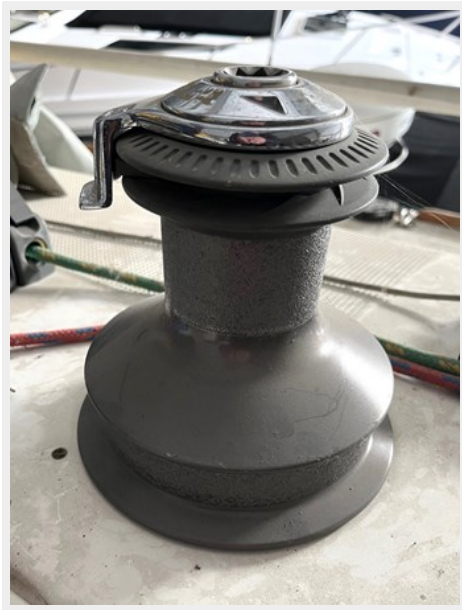
Pit winches - EVO Speed Ring drums IMG_2092
