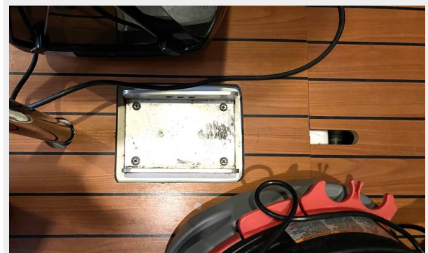
Mast step IMG_2125
