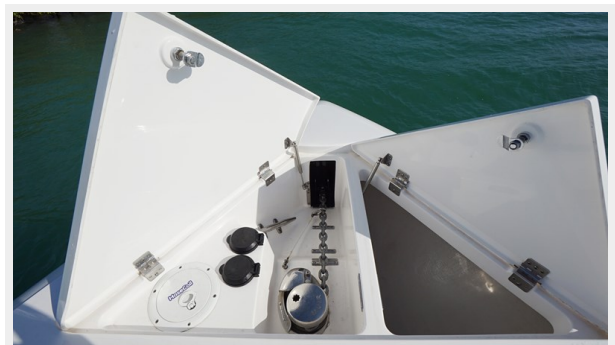
Windlass and Anchor Chain Locker
