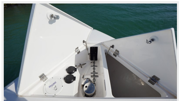
Windlass and Anchor Chain Locker
