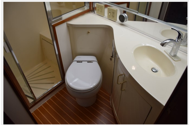
Head, New Techma Freshwater MSD
