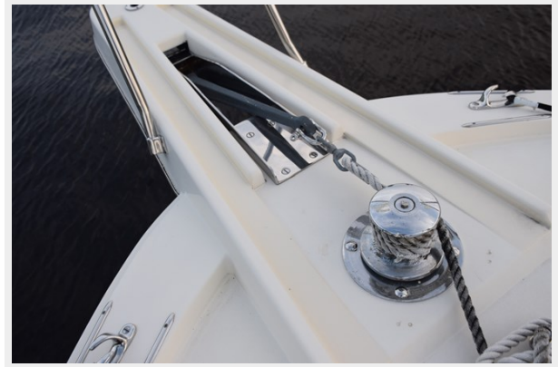
Rebuilt Galley-Made Windlass, CQR Anchor -Rode
