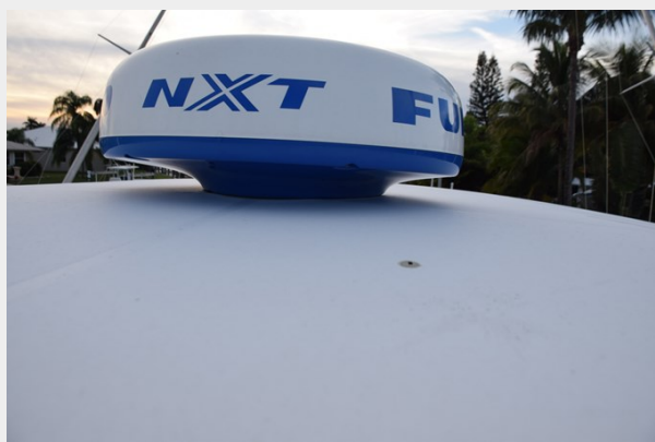
Doppler Solid-State 25w Radar
