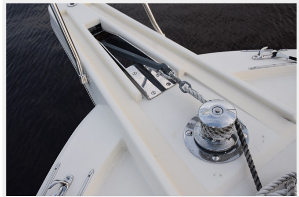
Rebuilt Galley-Made Windlass, CQR Anchor -Rode
