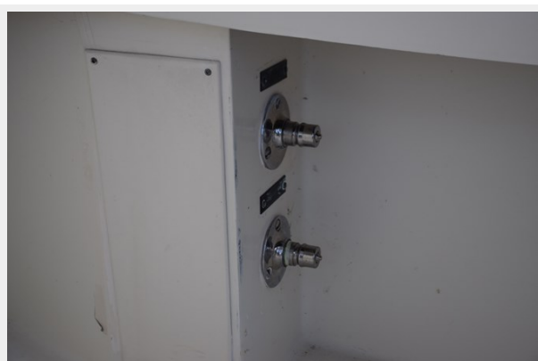
Quick Connect Cockpit Washdown Outlet and Shore Water Inlet
