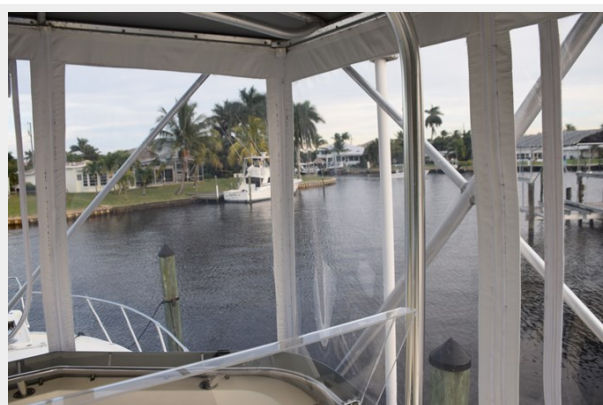
New Flybridge Enclosure
