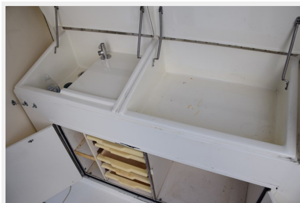
Tackle Center and Rigging Sink, New Faucet
