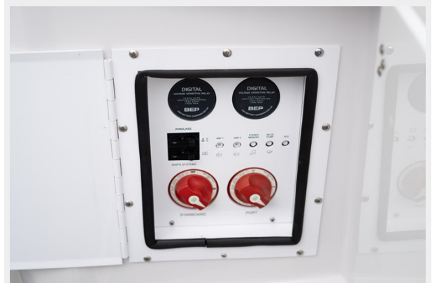
26. h290 battery switches
