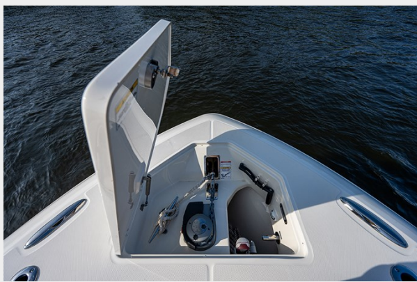
Bow anchor locker
