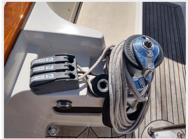
Phoenix electric winch and stoppers port
