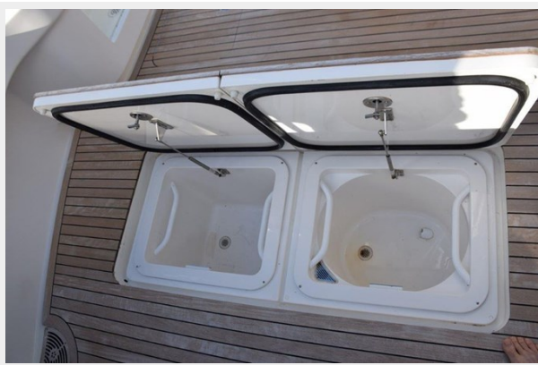
Below Deck Livewell and Storage Well, Starboard
