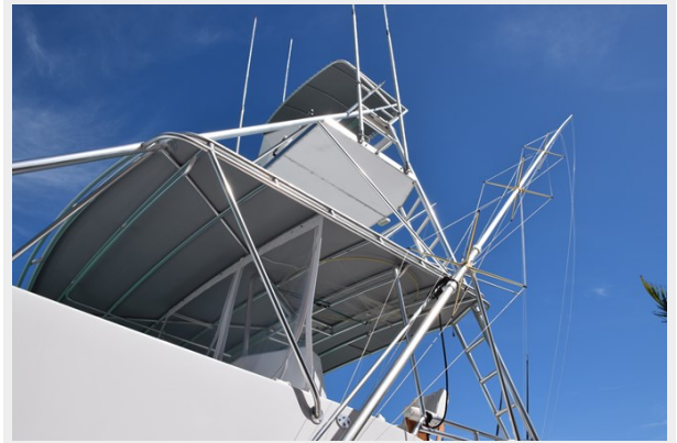
Tower with triple spreader outriggers
