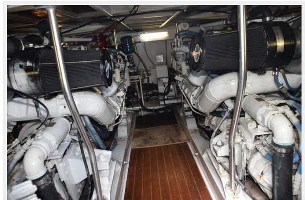
Engine room, Detroit Diesel 8v92s
