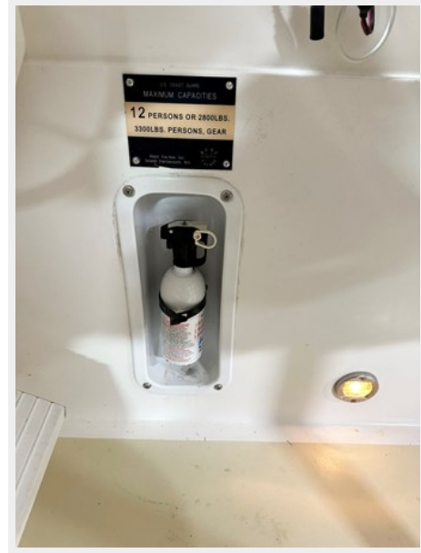
Fire Extinguisher Recessed Mount at Helm
