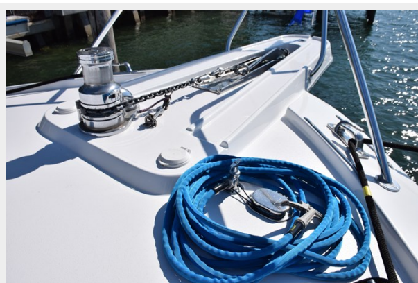
Anchor, Windlass, Washdown on Pulpit
