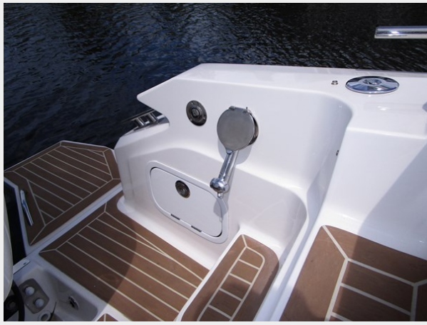
Port Stern Fresh Water Shower
