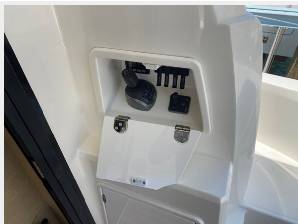
Joy stick and bow thruster controls on aft deck
