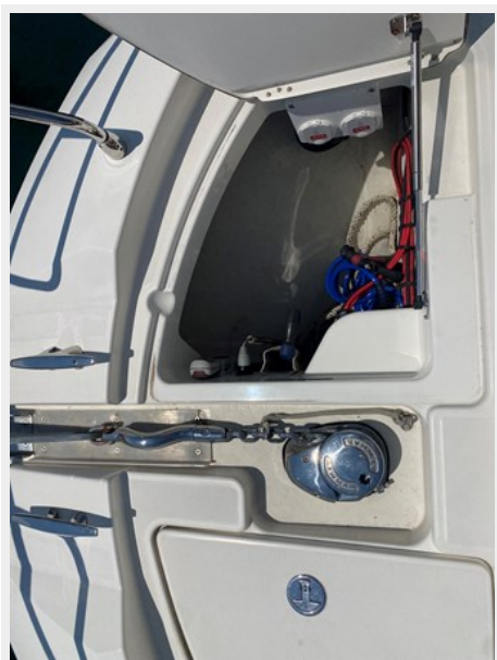
Anchor equipment on bow
