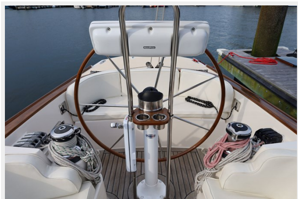
Steering Pedestal Looking Aft
