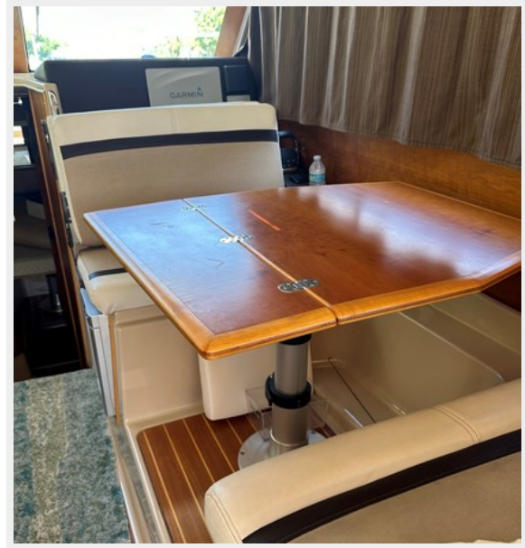
Dining table can be lowered and a cushion inserted to convert to a berth
