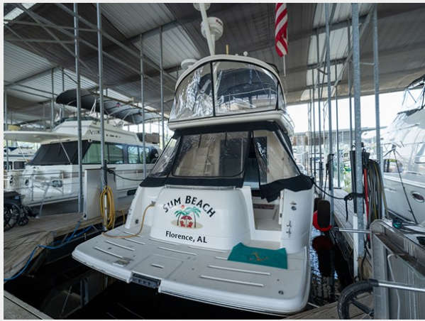
Swim platform (in slip)
