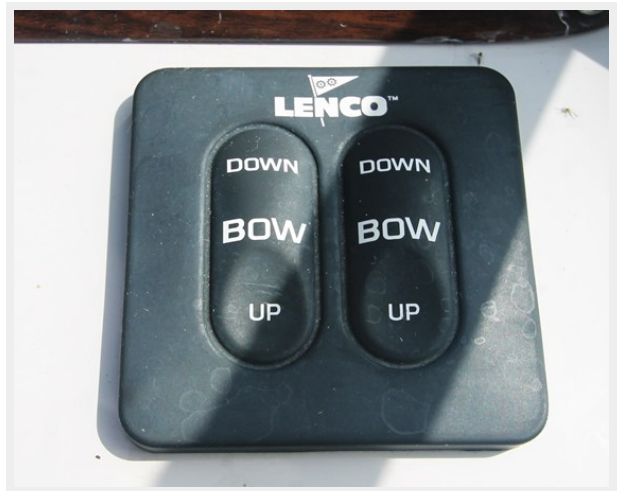
Trim Tab Controls
