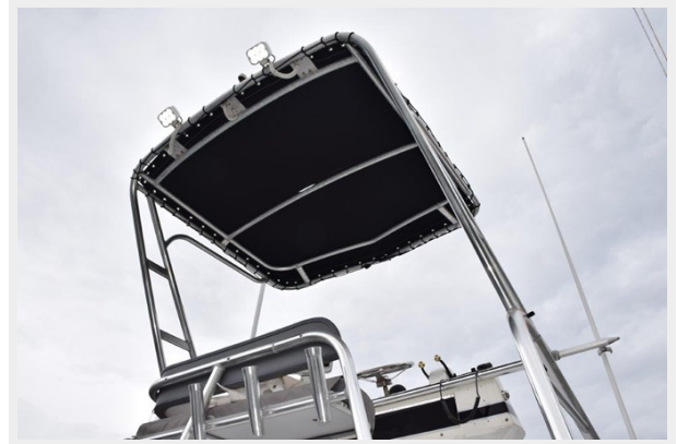
LED Spreader Lights, Open Side of Tower
