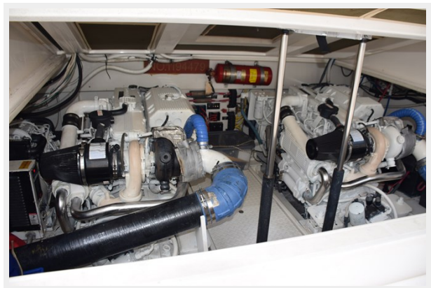
Cummins 540hp Common-Rail Diesels
