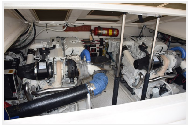
Cummins 540hp Common-Rail Diesels
