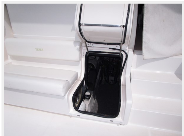
Cockpit Engine Room Access
