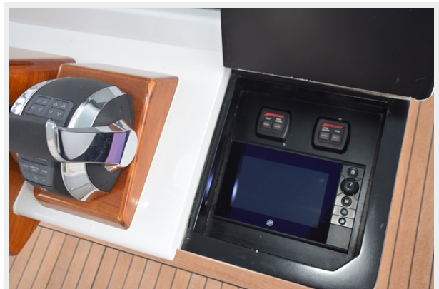
Mercury controls, start stops and display panel
