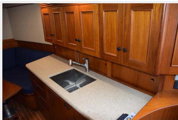
Corian countertop with stainless sink
