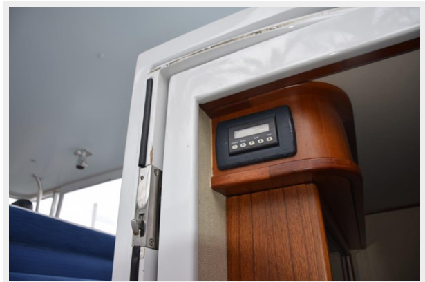
Bridge Deck A/C control and sliding cabin door
