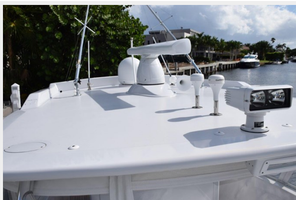
Hardtop antennas, spotlight and Rupp radial outriggers
