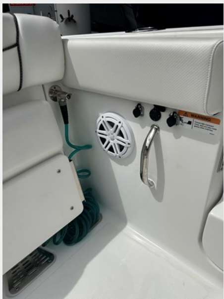
35. 302 wash down electric reel
