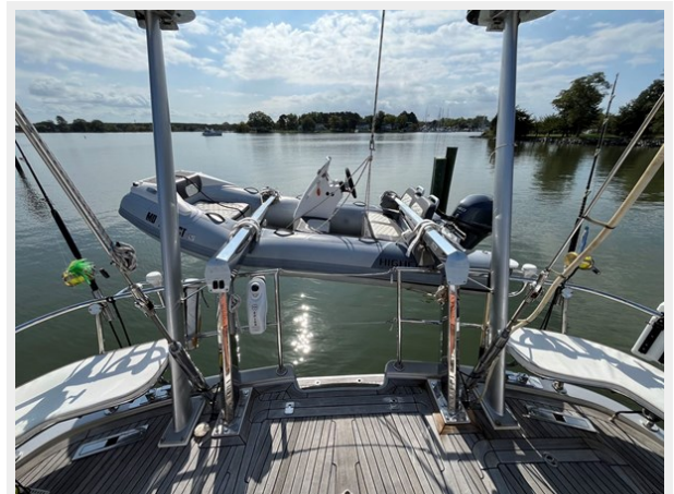
RIB in electric davits
