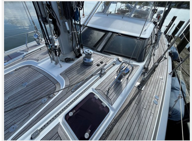
Port side electric halyard winch
