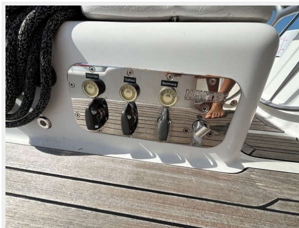
Navtec hydraulic panel
