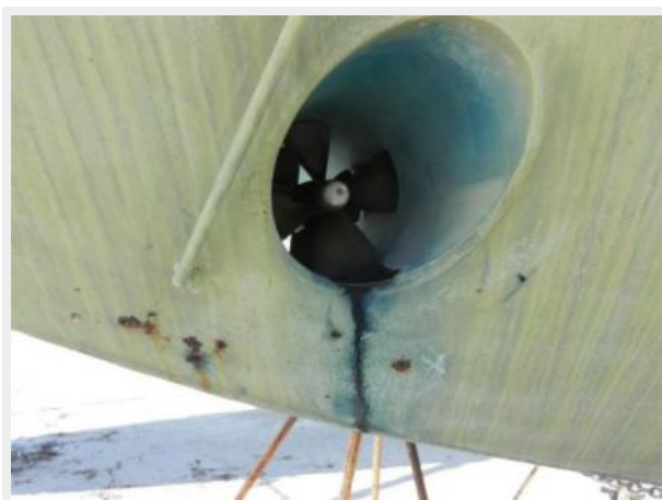
rust at concrete ballast at bow thruster
