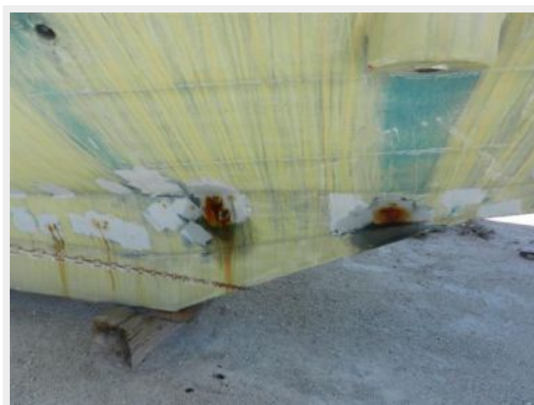
specific area of rust in keel where concrete ballast is located
