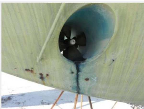
rust at concrete ballast at bow thruster
