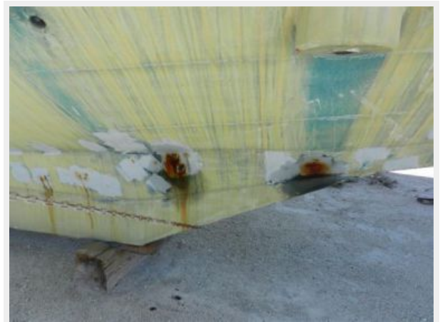
specific area of rust in keel where concrete ballast is located
