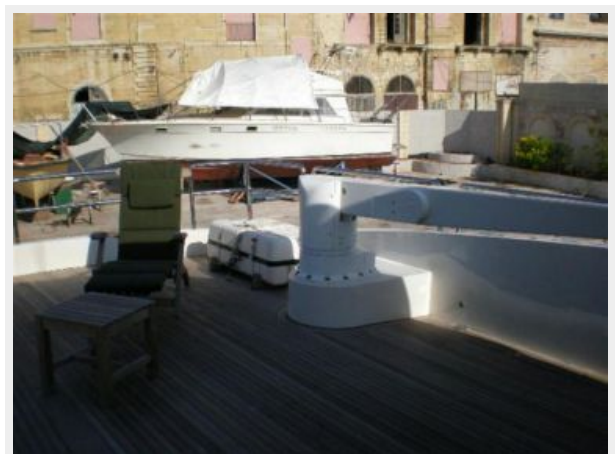
Upper deck showing tender crane
