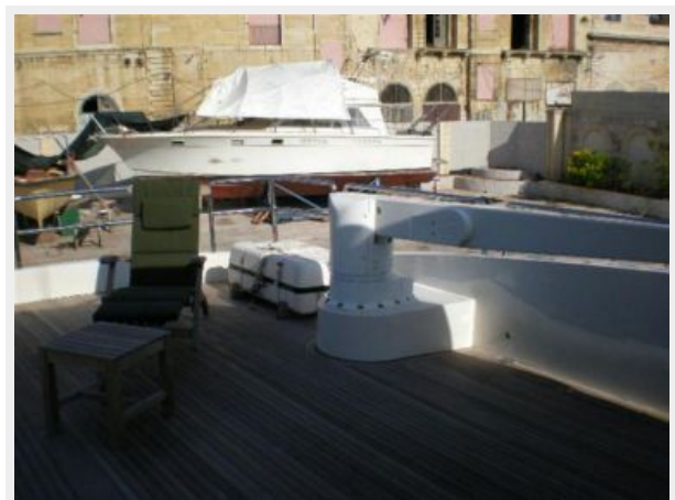
Upper deck showing tender crane
