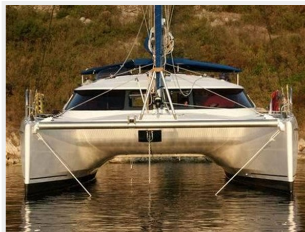
High Bridgedeck Clearance
