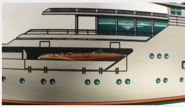
re-fit tender garage
