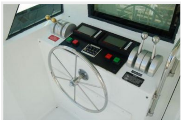
External helm controls
