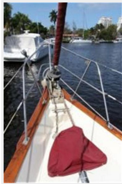
Bow with windlass and anchor platform
