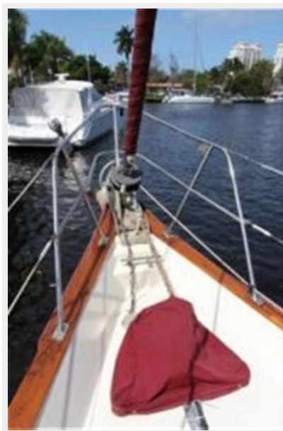
Bow with windlass and anchor platform
