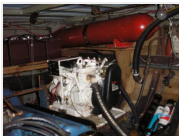
Onan Genset with Fire Suppression System
